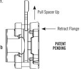
b) To remove water meter, remove bolts attaching flange to meter, pull spacer up out of groove and retract flange.
