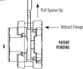
b) To remove water meter, remove bolts attaching flange to meter, pull spacer up out of groove and retract flange.
