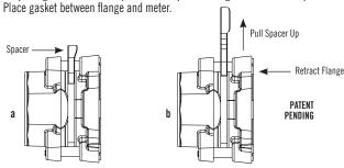
b) To remove water meter, remove bolts attaching flange to meter, pull spacer up out of groove and retract flange.
